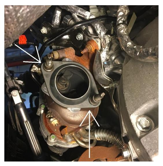
Step 5: If you're using the included stud socket, heat the turbo housing where the arrows are pointing to until red hot and then remove the studs. If you're using a heavy duty stud extractor like a Mac SR-10A socket, then not much heat is needed here.
