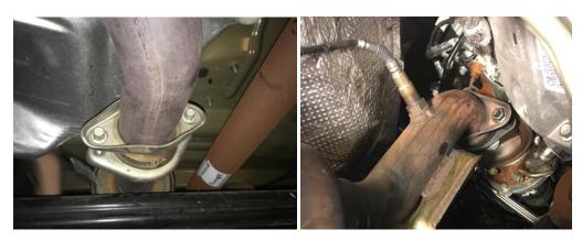
Step 3: Remove the two bolts that connect the downpipe to the resonator pipe.
